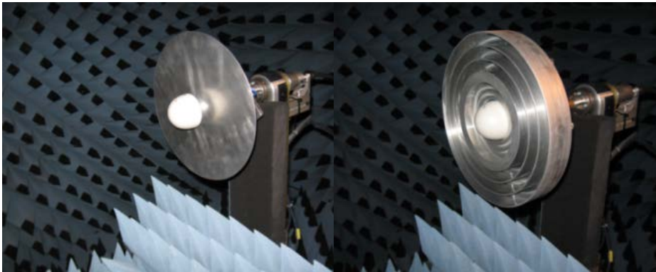
Calibration of TBIII antenna with flat Ground Plane and Choke Ring Ground Plane
