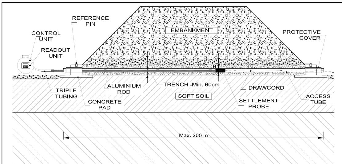
Figure 6. Schematic arrangement of the hydrostatic profile gauge
