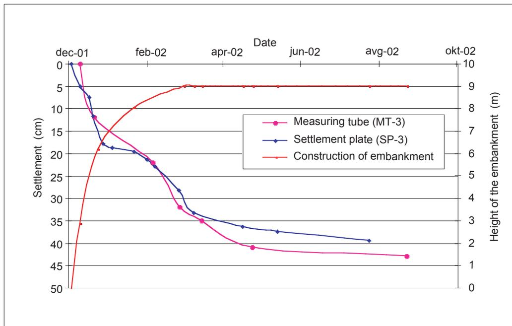
Figure 9. Settlement development measured using 2 different methods, compared to the progress of embankment construction
