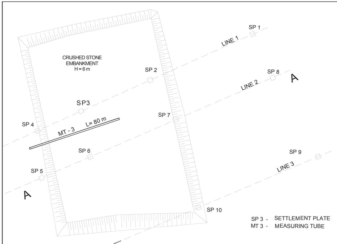
Figure 4. Field instrumentation of the embankment – plan
