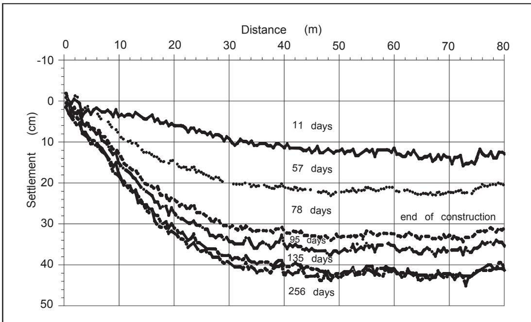
Figure 8. Settlement profiles at different times (since the 1st measurement) along the measuring tube MT-3
