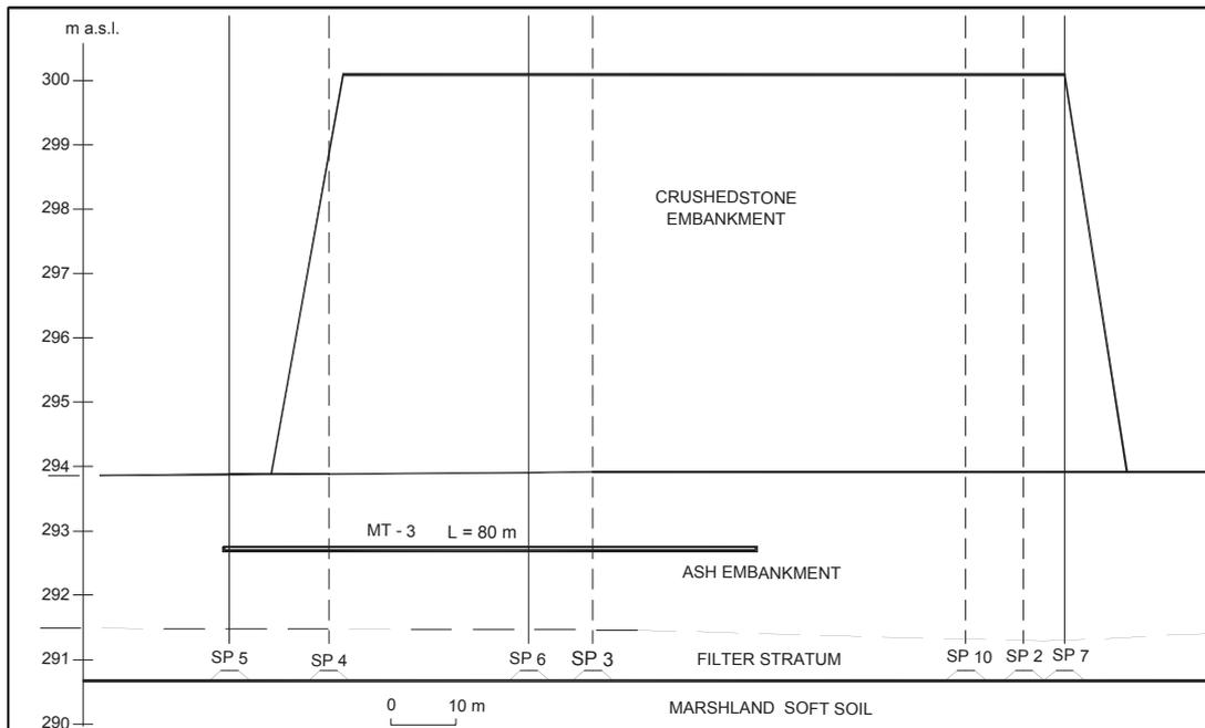
Figure 5. Field instrumentation of the embankment – cross section A-A
