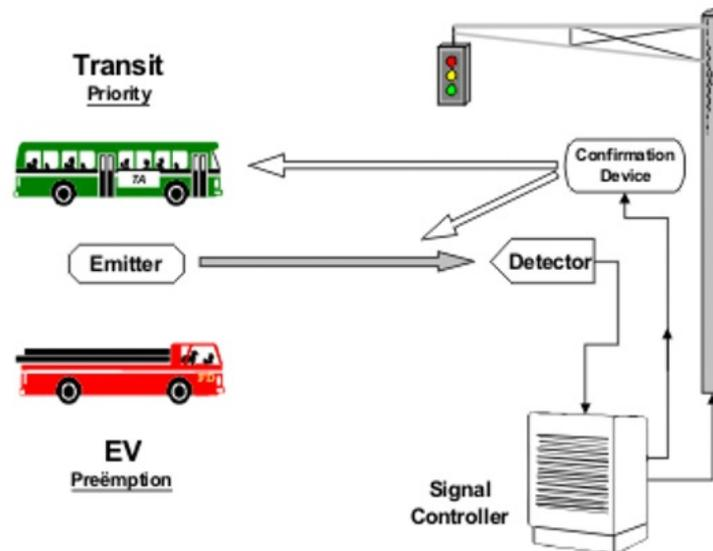
Fig 5. Vehicle detection and signal control in traffic lights.
