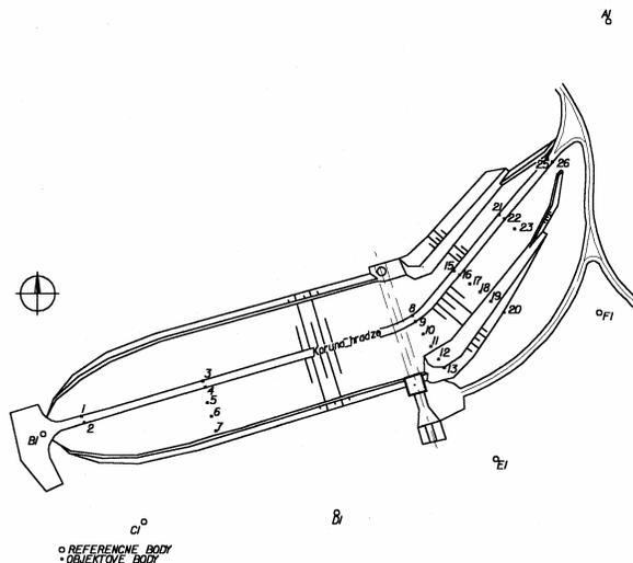
Figure 1b - The network point field of the bulk dam
