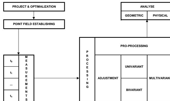
Figure 2 - Scheme of deformity detection algorithm
