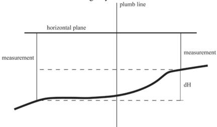
Figure 2. Geometric levelling
