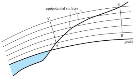
Figure 1. Non-parallelity of equipotential surfaces
