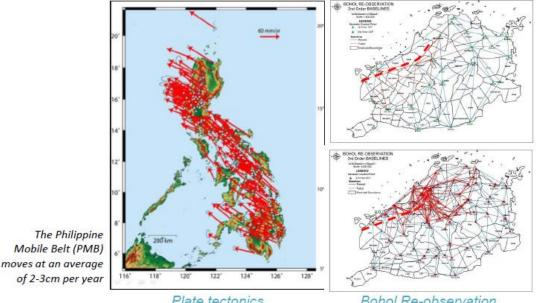
Re-observation of ground control points after the 2013 Bohol earthquake showed a maximum 2D displacement of 0.46m
