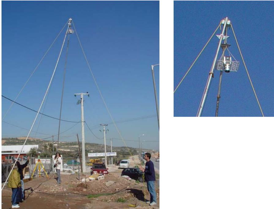
**Figure 4.** The bipod at the excavation area, during the field work.
