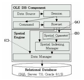
Picture 4 System Configuration of OGC OLE DB Component
