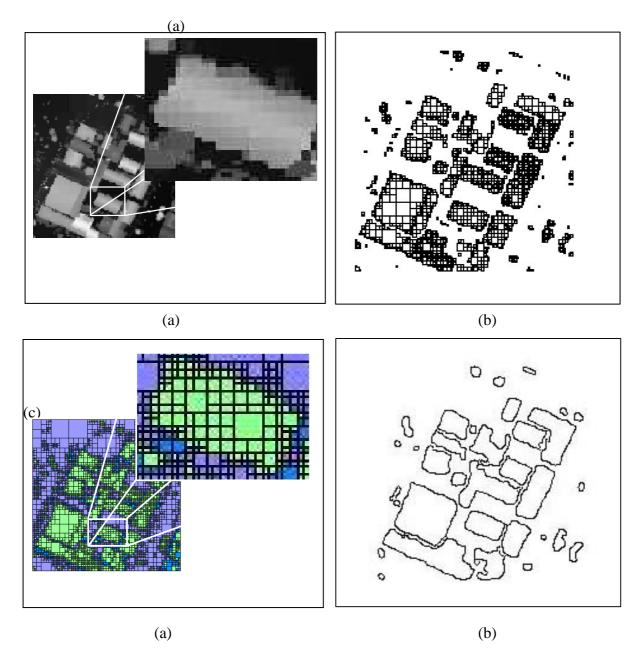
**Figure 5** – Result of the DEM segmentation using the proposed methodology. (a) Result of recursive splitting. (b)Contour obtained by the recursive splitting. (c) Region merging result (d) Contour obtained by region merging.
