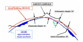
**Figure 1.** Relationship between ellipsoidal and orthometric heights (http://www.usace.army.mil/usace-docs/eng-manuals/em1110-1-1003/c-3.pdf, accessed February 2006
