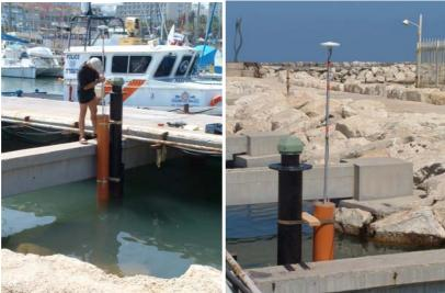
Figure 3 – GPTG installed near the traditional SOI-TG.
