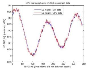
Figure 4 – Comparison of SOI-TG data versus the GPS mariograph data.
