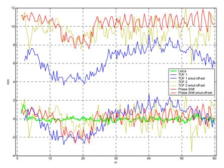
Figure 8: Differences between and the interferometer and the four EDM sensors
