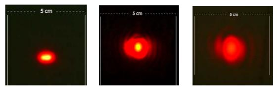
Figure 10: Leica's laser spot size at distance: 5, 35, and 55 m
