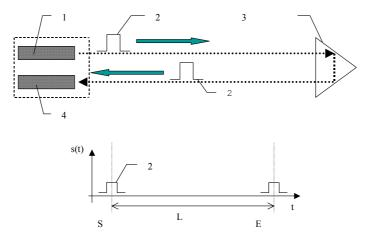
Figure 5: The principle of the transit time method
