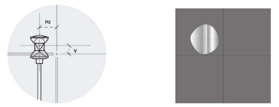
Figure 2: ATR's Hz and V offsets, and the prism's image on the CCD chip
