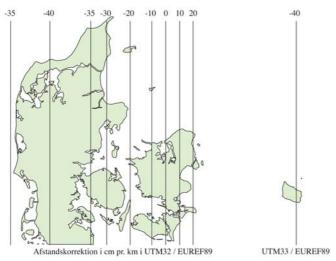
**Fig. 1** UTM32 and UTM33/ETRS89. Distance correction in cm/km
