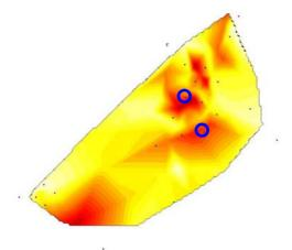
**Figure 6:** The variations of deformations of the local control network of Tranås, based on the residuals shown in figure 5. The deformations are weighted inversely to the square of the point distance. The two marked common control points were deviant, and finally excluded.
