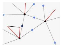
**Figure 4d:** The d value is moved to the middle point of the triangle side. The same procedure is carried out for all triangle sides of the triangulation. Figure 6 shows a Matlab plot of these d values.
