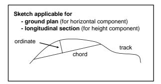
Fig. 8: Ordinates with respect to the chord according to Nalenz-Höfer procedure
