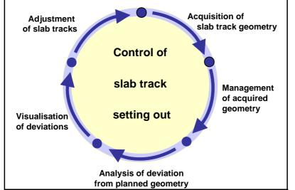
Fig. 4: Construction circle integrated into construction of "Feste Fahrbahn"
