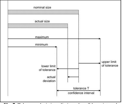
Fig. 7: Tolerance, deviations, limits and confidence interval
