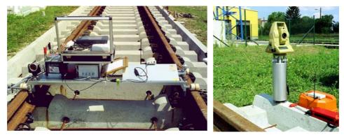
Fig. 10: Track measuring vehicle and tachymeter on special pillar
