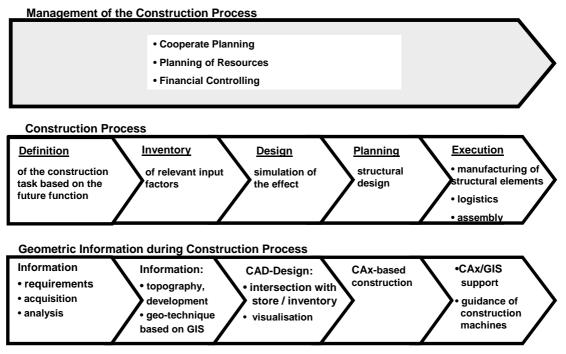
Fig. 1: Construction process and required information input
