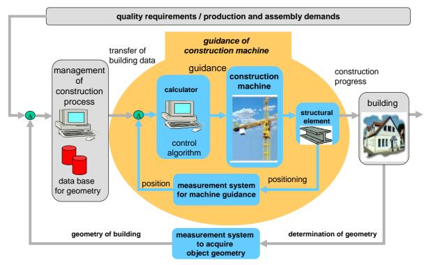
Fig. 11: Quality driven control circles for the construction process
