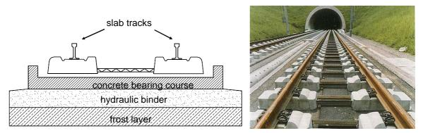
Fig. 3: Slab track construction "Feste Fahrbahn" (principle and example picture)
