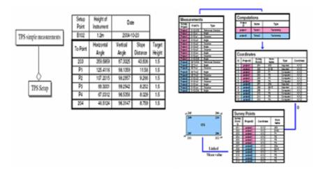
Figure 3.4 Data Model of TS Surveying Results
