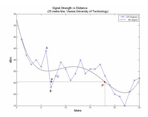
Figure 6: Illustration of incorrect SS to distance conversion based on curve fitting
