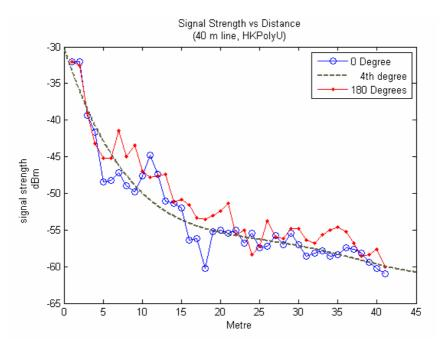
Figure 4: Test result of signal strength vs. distance over a 40 metre baseline in HKPolyU
