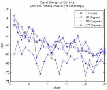
Figure 5 (a): Test result of signal strength vs distance over a 25 metre baseline at TU Vienna
