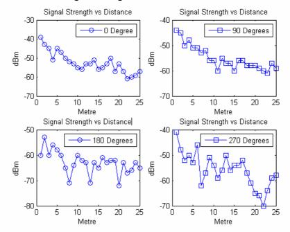
Figure 5 (b): 25 metre baseline test at TU Vienna: Plot of data collected in the directions 0°, 90°, 180° and 270°
