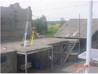
Picture 2. DPT-base station on a temporary fix point in the field office of the surveying squad
