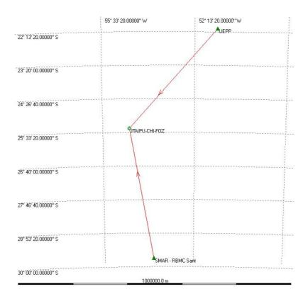
Fig 3: Vectors to be processed and adjusted for ITAIPU-CHI-FOZ station
