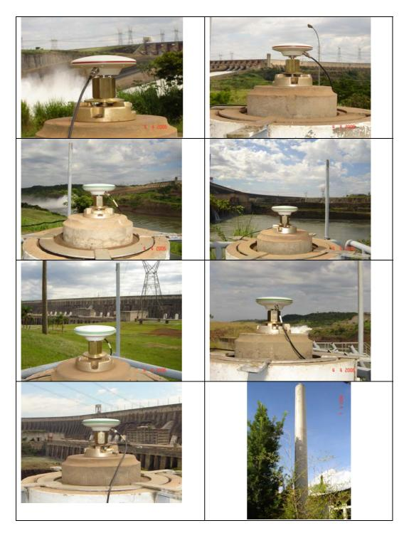
**Fig 2**: Installation of GPS Antennas on top of pillars P1 to P7 and the fix Station ITAIPU-CHI-FOZ respectively
