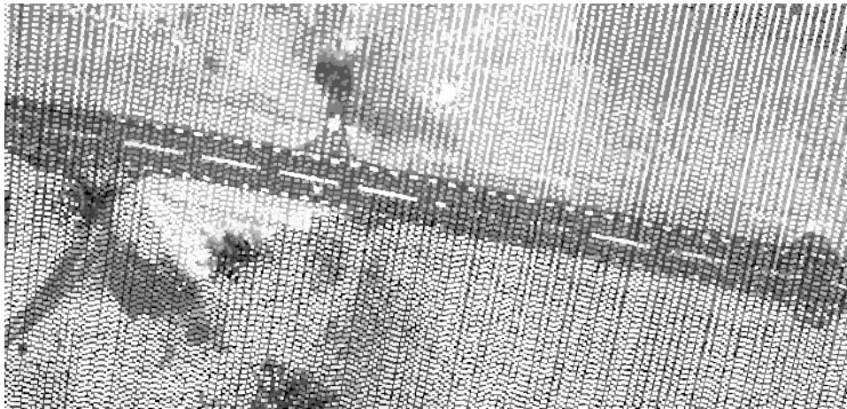
Figure 2.3 Planimetric control can be derived to the intensity of laser data, e.g. painted details on the roads. These can also be used as control of orthophoto.
