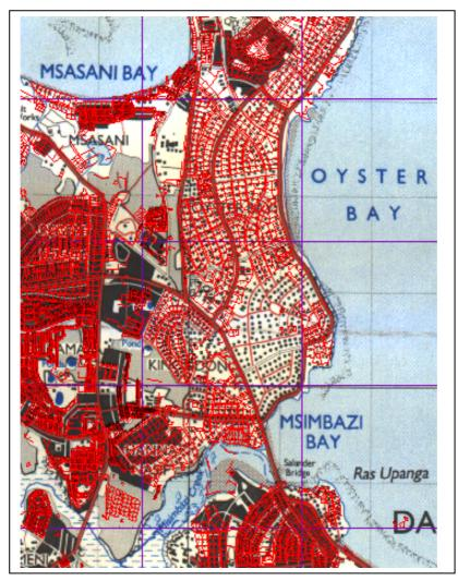
The Cadastral survey image on the Topographical Map will play a vital role for locating the new surveys submitted for approval in order to identify block and plot numbers and to prevent overlaps with old surveys. But the technique requires field work in case the new survey is in local coordinate system.
