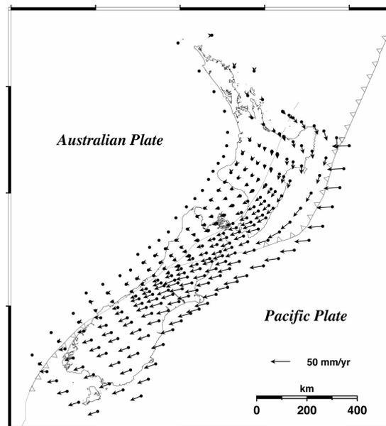
**Fig 5:** GNS deformation model showing horizontal velocities (Beavan 1998).
