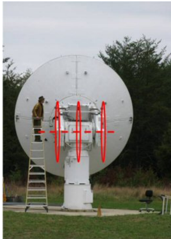
Figure 11: Determination of Elevation Axis for VLBI
