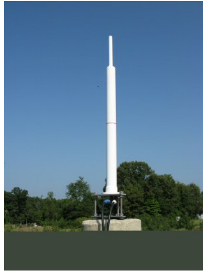
Figure 5: The DORIS antenna at GGAO
