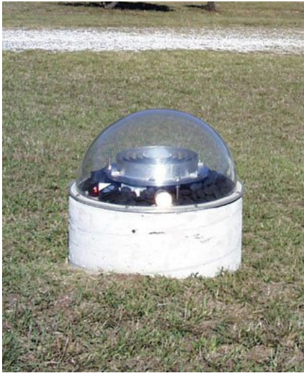
Figure 4: The GPS antenna (GODE) at GGAO (Photo courtesy of NASA)
