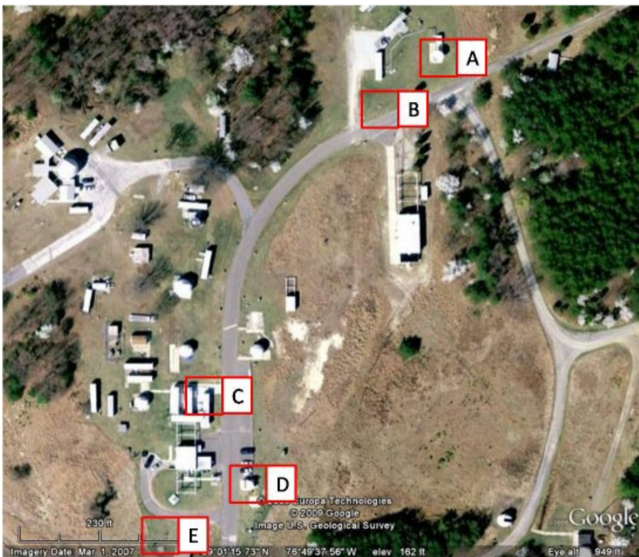
Figure 6: Plan view of GGAO showing the four space geodetic techniques: (A) VLBI, (B) GPS (GODE), (C) SLR/MOBLAS-7, (D) SLR/NGSLR, (E) DORIS
