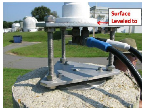
Figure 8: Surface to which geodetic leveling was taken at DORIS antenna.
