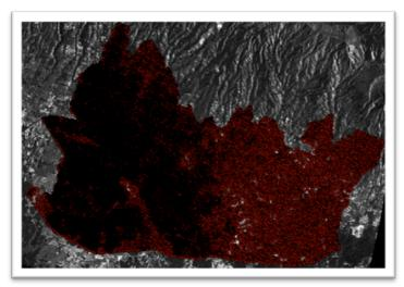
Figure 3. PS points density distribution of PS-InSAR processing in Bandung city area.
