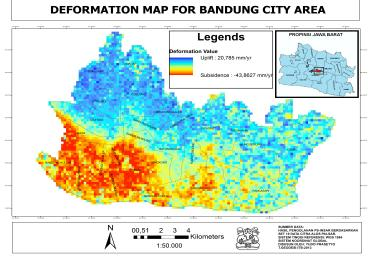
Figure 4. Deformation map from PS-InSAR processing in Bandung city area.
