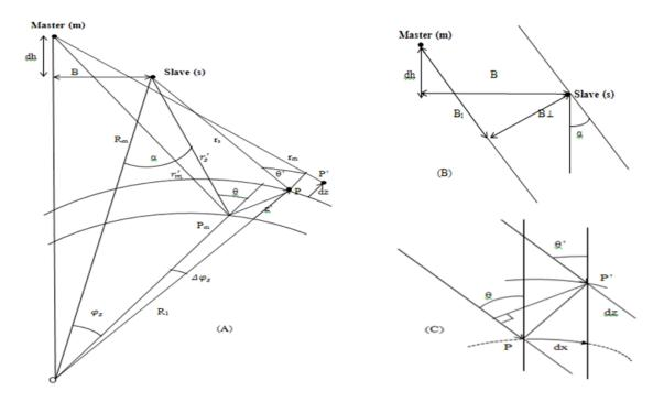
Figure 2. Radar geometry for earth surface deformation (Sumantyo et al., 2009)
