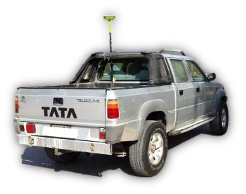
Figure 4 Receiver (Rover) Located on the Car
