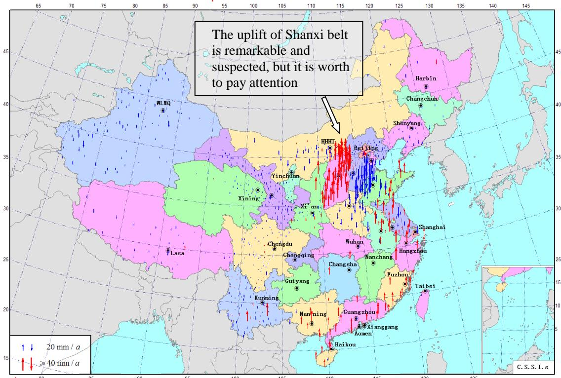
Figure 8 Vertical deformation field from GNSS (2004-2007)
