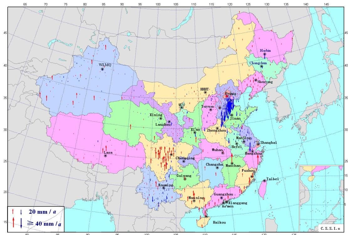
Figure 5 Vertical deformation field from GNSS(1999-2004)
