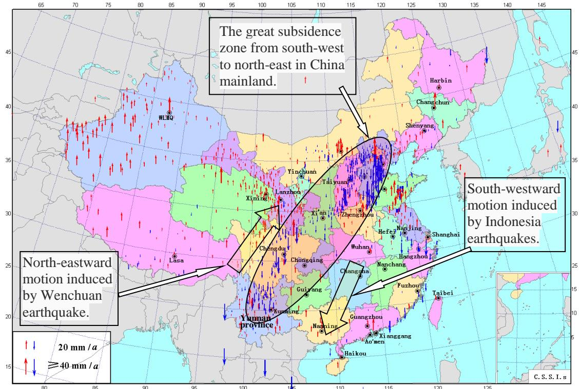
Figure 7 Vertical deformation field from GNSS (2007-2009)
