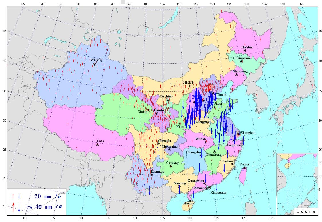
Figure 3 Vertical crust deformation shown by regional GNSS
