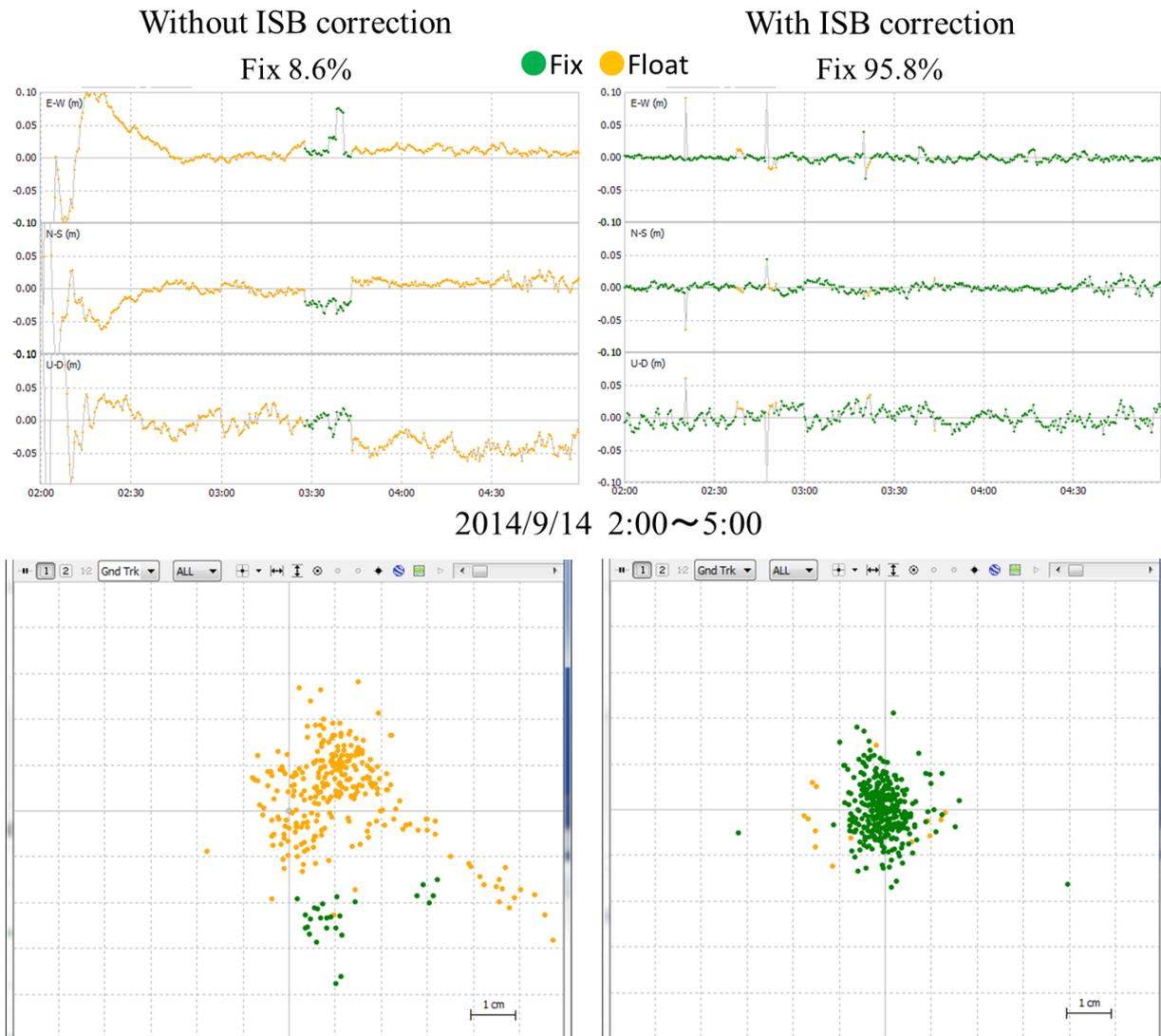
Fig.14: GPS and Galileo kinematic solutions of 500 m baseline at GSI in Tsukuba on September 14, 2014, between JAVAD DELTA and Trimble NetR9 receivers. Ambiguities between GPS and Galileo are successfully resolved with ISB correction of Phase L1 0.042m and Phase
