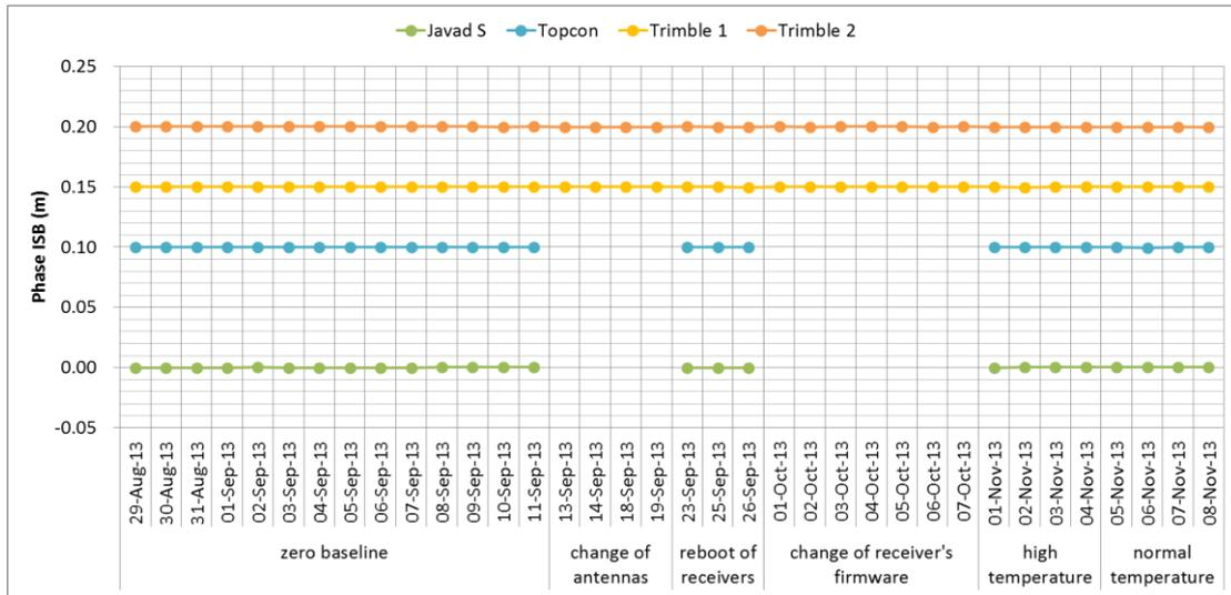
Fig.7: Variations of L1 ISB of GPS-QZSS with respect to JAVAD DELTA receiver
