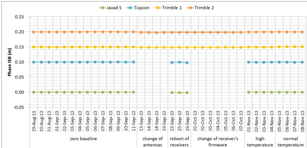
Fig.8: Variations of L2 ISB of GPS-QZSS with respect to JAVAD DELTA receiver
