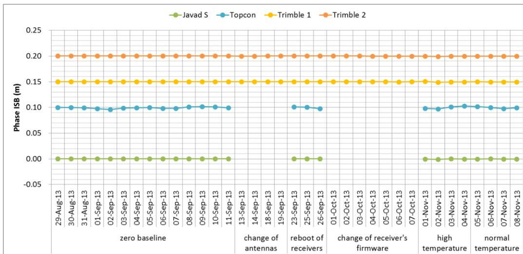
Fig.9: Variations of L5 ISB of GPS-QZSS with respect to JAVAD DELTA receiver
