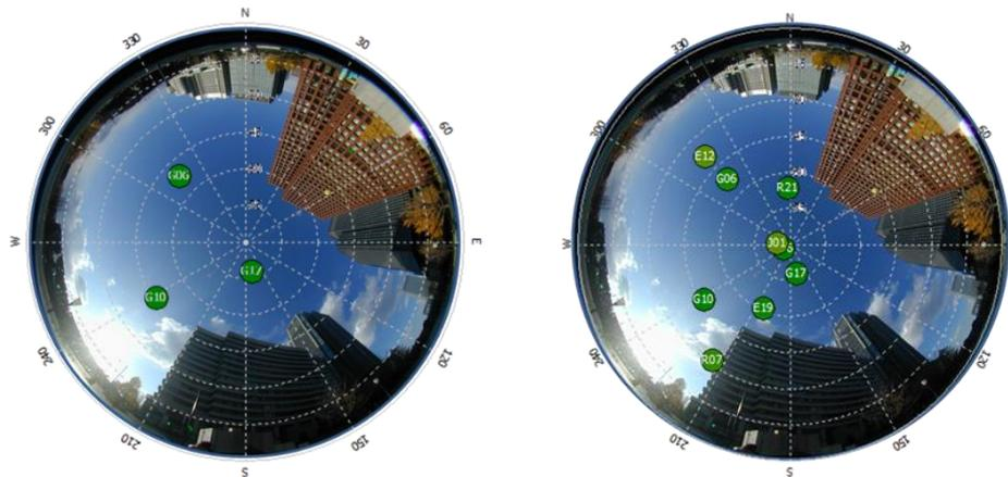
Fig.2: An example of satellite visibility in an urban canyon of Tokyo, at 1:00 UTC December 14, 2014. Left: No hope of positioning with only 3 GPS. Right: Positioning possible with additional 1 QZSS, 3 GLONASS, and 2 Galileo.
