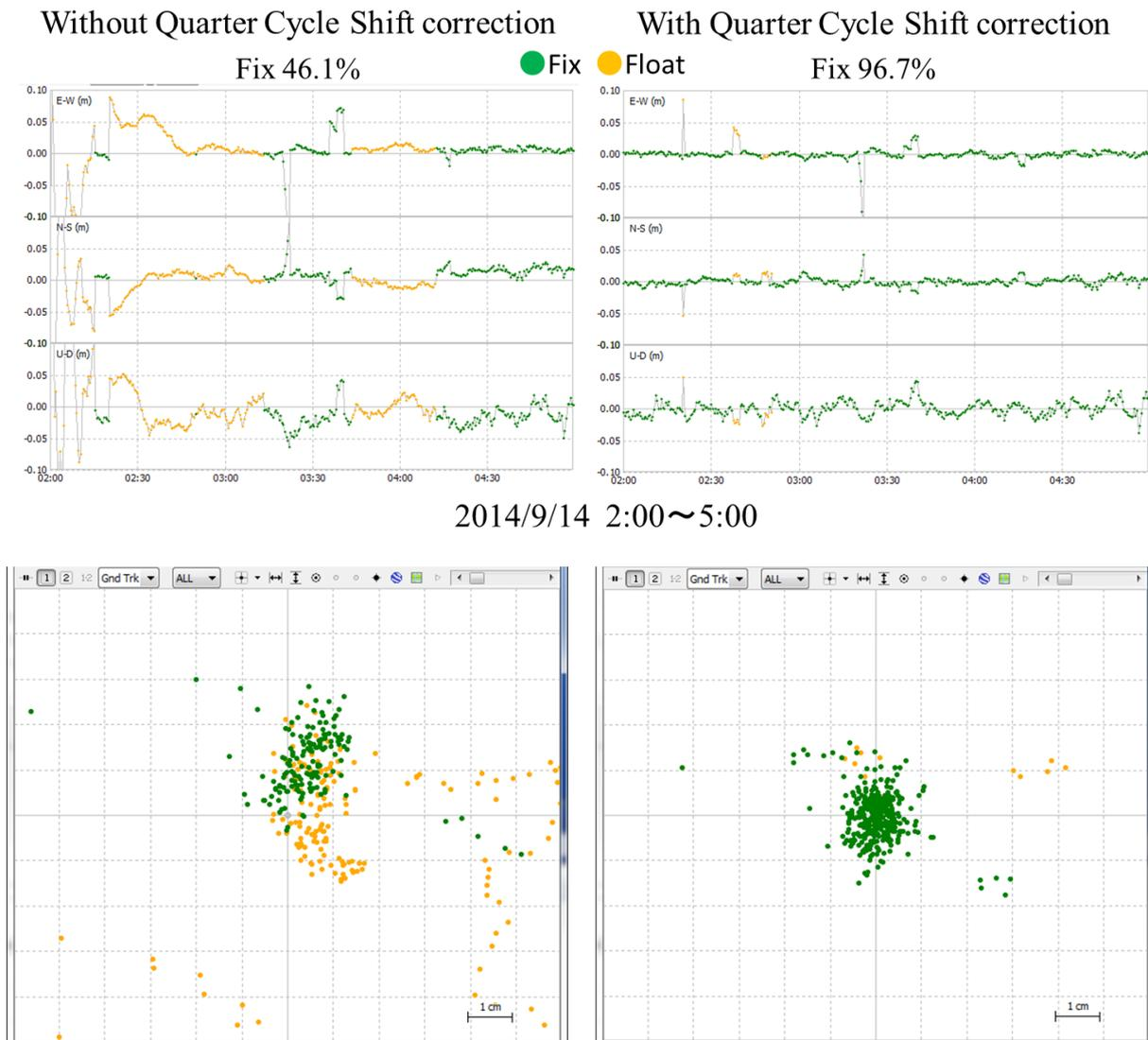
Fig.6: GPS and QZSS kinematic solutions of 500 m baseline at GSI headquarters in Tsukuba on September 14, 2014, between JAVAD DELTA and Trimble NetR9 receivers. We previously
