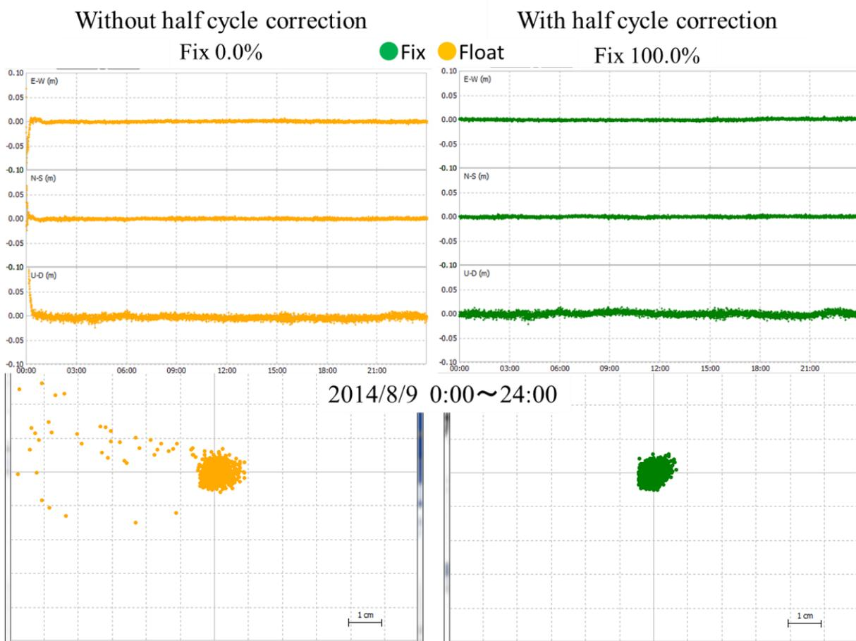
Fig.15: GPS and BeiDou kinematic solutions of a zero baseline at Etchujima, Tokyo on August 9, 2014, between JAVAD DELTA and Trimble NetR9 receivers. Unit for vertical axis of upper graphs is meter.
