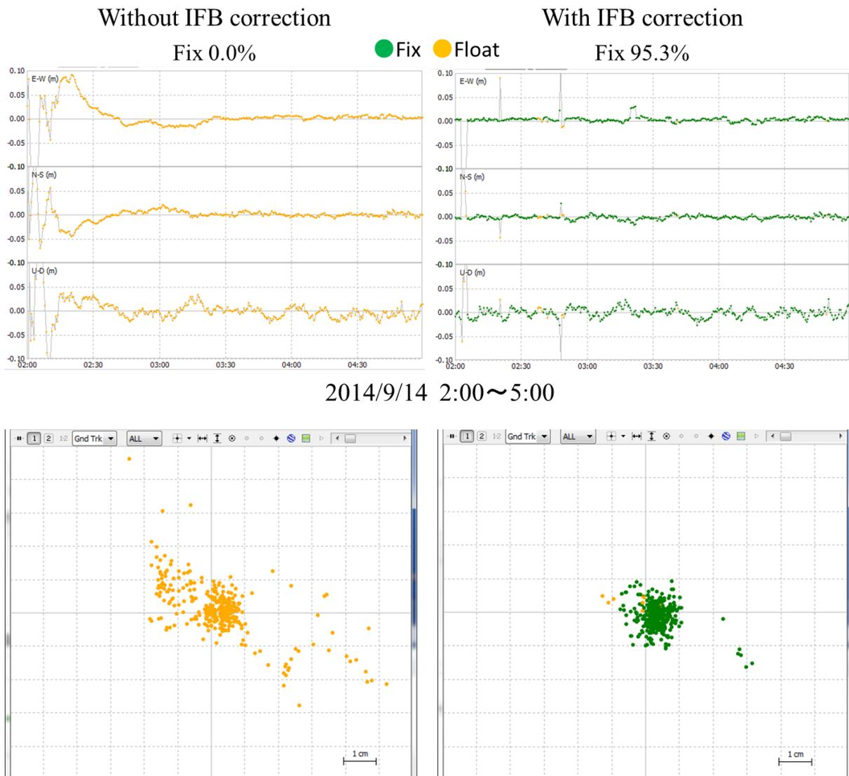
Fig.5: GPS and GLONASS kinematic solutions of 500 m baseline at GSI headquarters in Tsukuba on September 14, 2014, between JAVAD DELTA and Leica GR25 receivers. IFB corrections applied for the GSILIB processing are 3.00 cm/Freq for L1 and 3.00 cm/Freq for L2 which are estimated from the zero baseline observation of 12 hours on August 27, 2014. Unit for vertical axis of upper graphs is meter.
