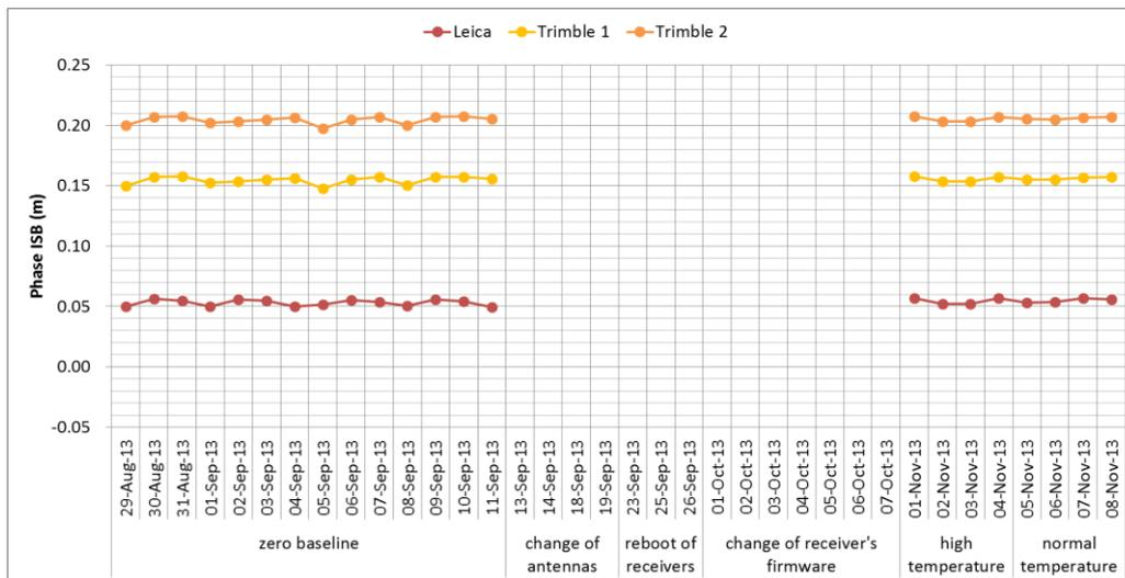
Fig.13: Variations of L5 ISB of GPS-Galileo with respect to JAVAD DELTA receiver
