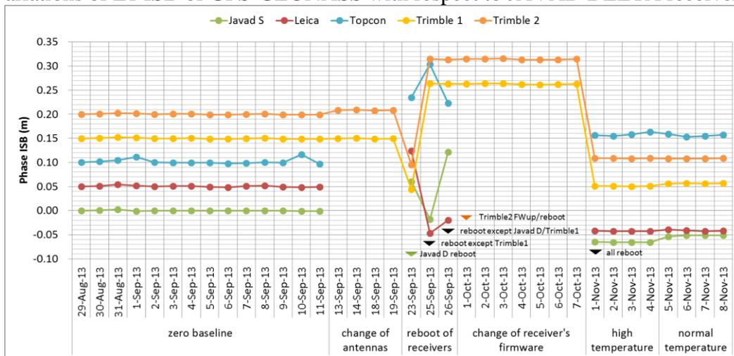
Fig.11: Variations of L2 ISB of GPS-GLONASS with respect to JAVAD DELTA receiver
