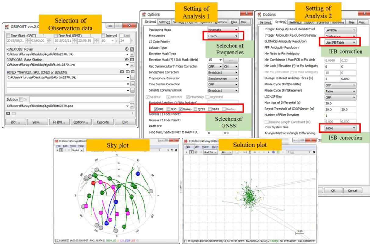
Fig.16: Interface and output view of GSILIB. GSILIB is a derivation from RTKLIB specialized in dealing with biases in multi-GNSS surveying.
