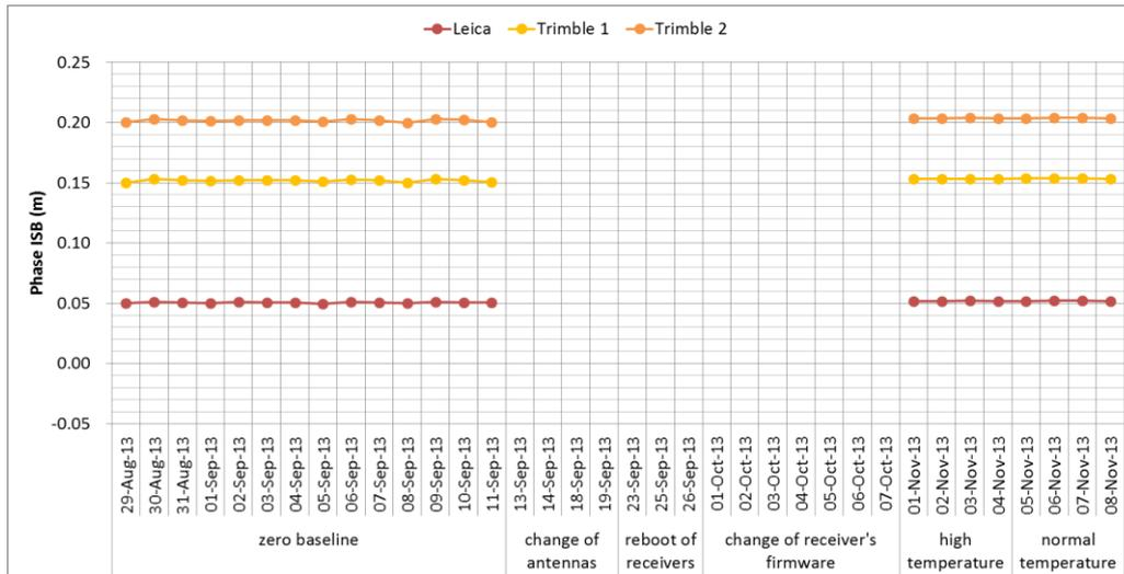
Fig.12: Variations of L1 ISB of GPS-Galileo with respect to JAVAD DELTA receiver
