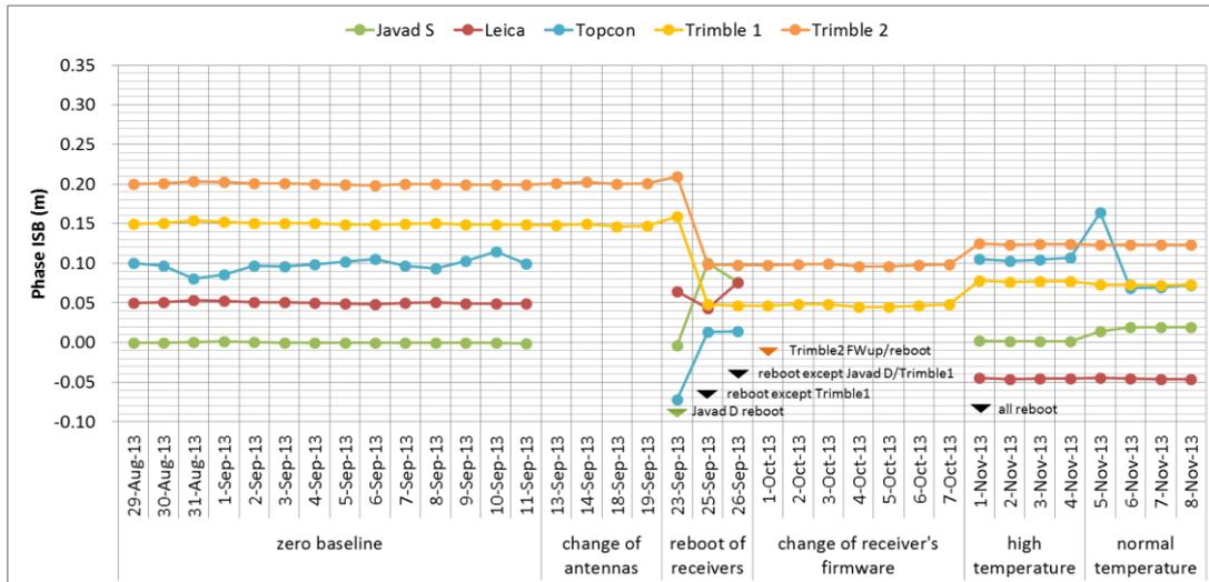
Fig.10: Variations of L1 ISB of GPS-GLONASS with respect to JAVAD DELTA receiver
