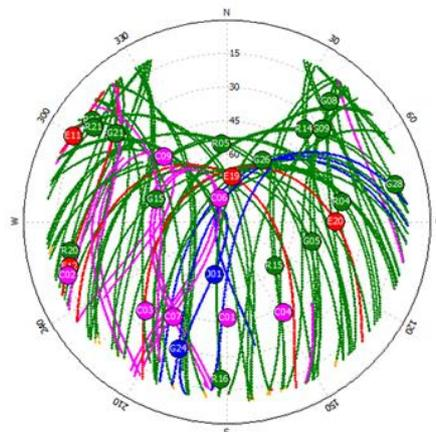
Fig.1: Sky plot of GNSS data observed by modern GNSS receiver (Trimble NetR9) at GSI headquarters in Tsukuba from 5:25 to 23:15 UTC on July 17, 2013. G: GPS, J: QZSS, R: GLONASS, E: Galileo, C: BeiDou.
