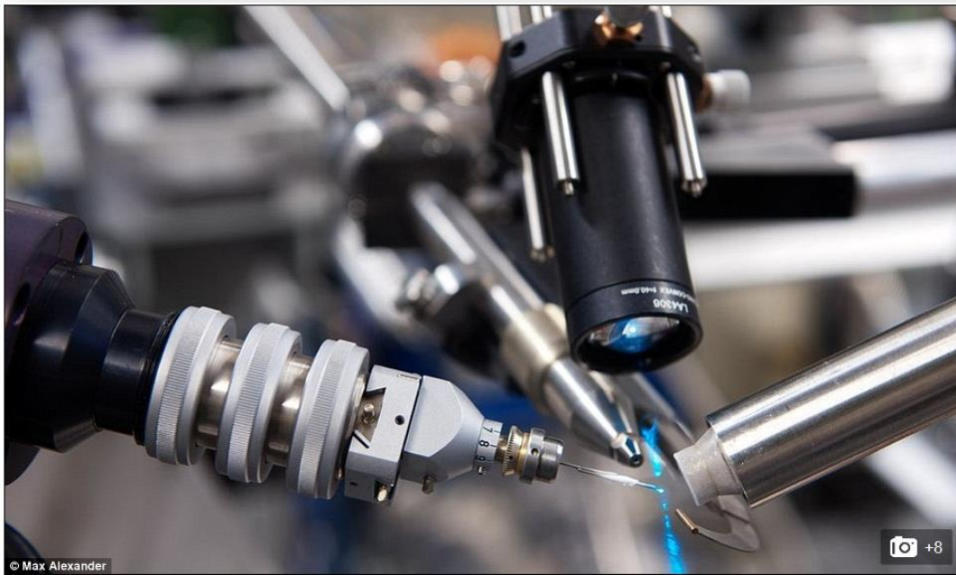
A crystal is placed on the end of the pin with a stream of cool air coming in from the right. The X-ray beam arrives from the silver pipe and the camera images the crystal
