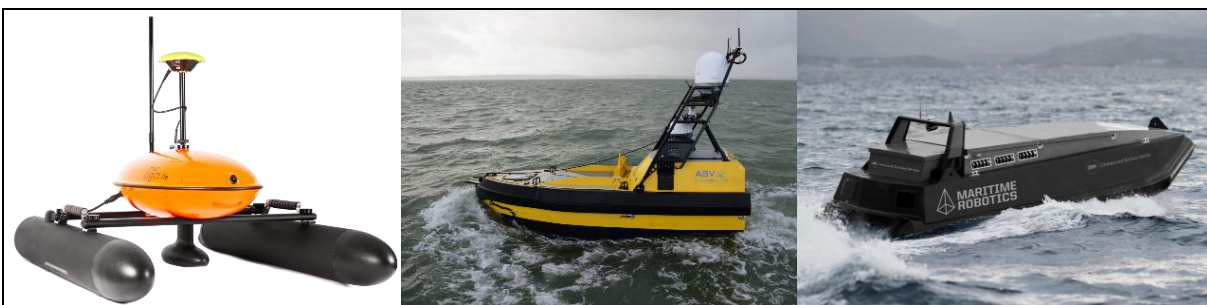
Figure 2: Unmanned surface vehicles of different sizes. From left to right: SONOBOT from EvoLogics ( www.evologics.de ), C-Worker 6 from ASV ( www.asvglobal.com ), Mariner from Maritim Robotics ( www.maritimrobotics.com ).
