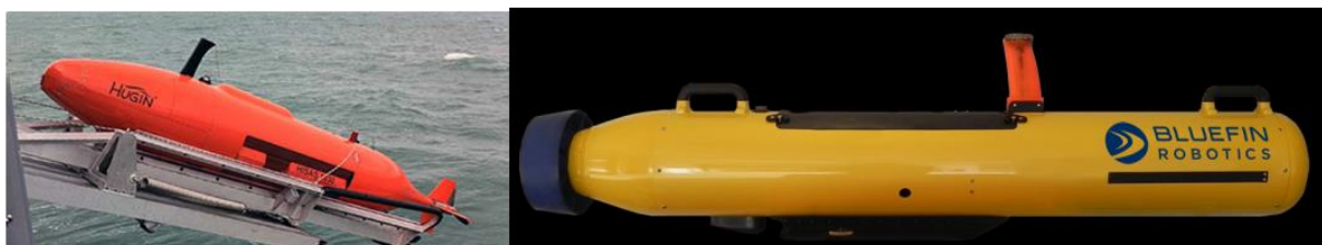
Figure 3: Unmanned underwater (or hybrid) vehicles. From left to right: HUGIN from Kongsberg ( www.kongsberg.com ), Bluefin-9 from Bluefin Robotics ( www.bluefinrobotics.com ).
