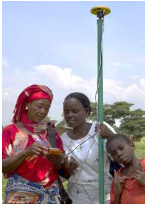
Two community members learning how to become para-surveyors using a smartphone and an external GNSS antenna to increase the positional accuracy in Luberizi, South Kivu, Democratic Republic of Congo.
