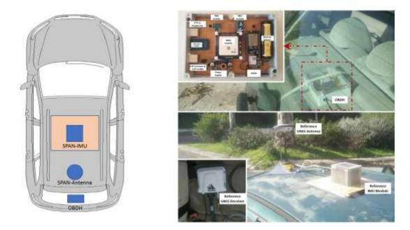
Fig. 4: Sensors setup during assessment trajectory data collection
