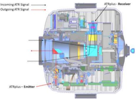
Figure 3 Optical path of ATRplus signals inside the TM60 telescope
