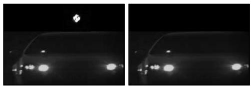
Figure 4 Bright (left) and dark (right) ATRplus image of a car and a reflective prism
