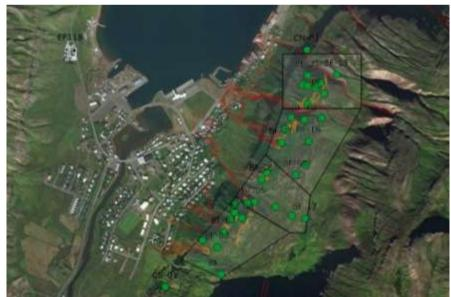
Figure 9 Monitoring system in Seyðisfjörður. EF118 is the location of the total station, while green dots represent the prisms. Red lines depict the outlines of the December landslides.
