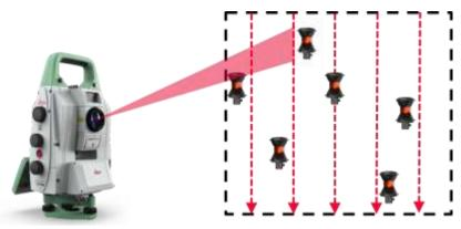
**Figure 5** Leica TM60 conducting the prism search within a defined area. The configuration was done using GeoMoS AutoLearn feature.
