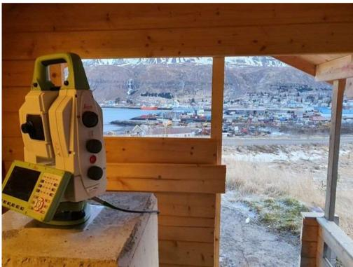
Figure 10 Leica TM60 I monitoring total station in the measurement hut
