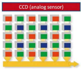
Principle of the interline transfer of CCD sensor A/D conversion outside of the sensor **Complementary Metal-Oxide Semiconductor, CMOS**
