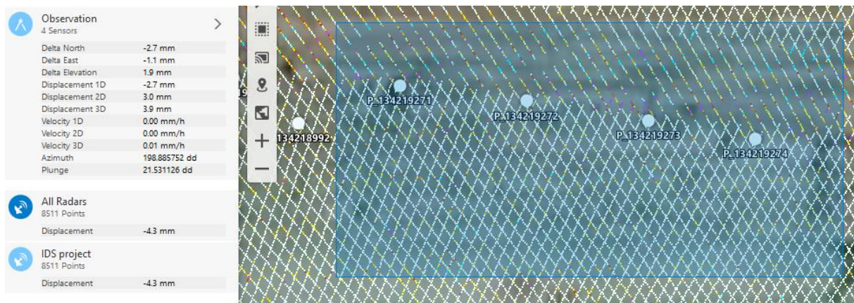
Figure 8 Cross-analysis of prism and radar monitoring data
