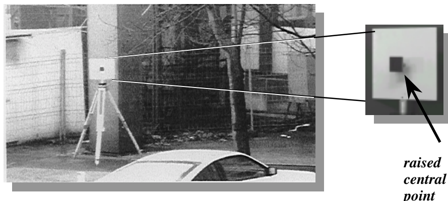
Figure 5: Three-dimensional target for calibration, sensitive towards distance-change and differences in contrast
