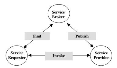
Figure 3: Web services architecture (Nagappan et al., 2003)
